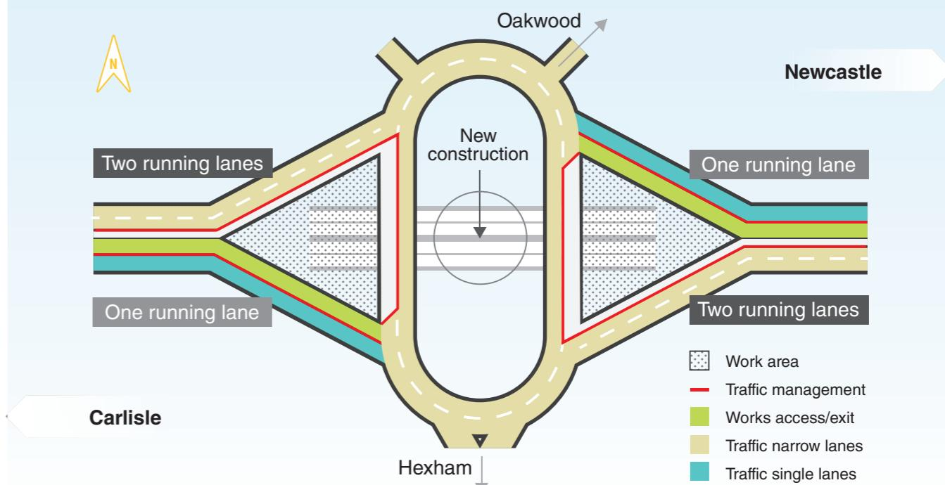
Two lanes will be used to approach the roundabout from Newcastle, with one lane dedicated to turning into Hexham and the other for turning right or through traffic. There'll be a short stretch of one lane open heading from Hexham towards Carlisle to allow contractors safe access to our work site.
